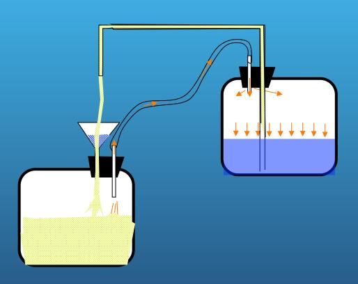
When water reaches the tube in the bottom stopper, flow of gas stops and fountain stops.
